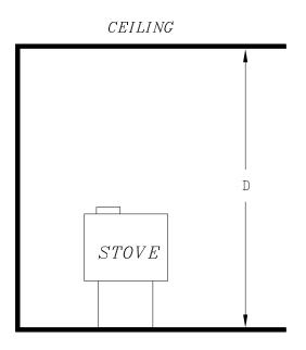
Figure 1.3 Clearances to combustible materials
